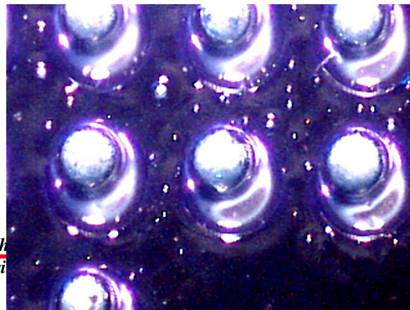
After Spreading Solder Paste into holes and heating to form Solder Balls
