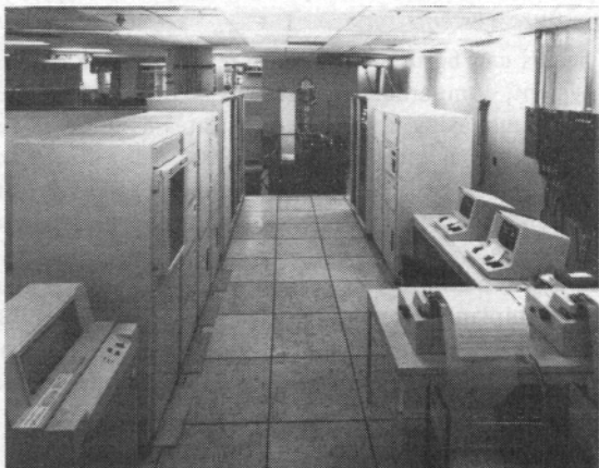
Fig. 5. The IBM EL-3 system is used for fast turnaround in electron-beam patterning of prototype devices.
