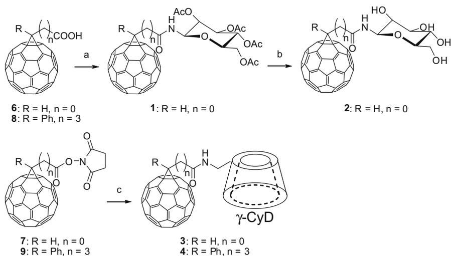
**Scheme 1.** Syntheses of  $C_{60}$  derivatives **1–4**. Reagents, conditions, and yields: (a)  $\beta$ -D-glucopyranosylamine 2,3,4,6-tetraacetate, EDCI, HOBT, DMF, 27–45%; (b)  $K_2CO_3$ , MeOH/ $CHCl_3$ , 76%; and (c)  $NH_2$ - $\gamma$ -CyD, DMF, 78–80%.
