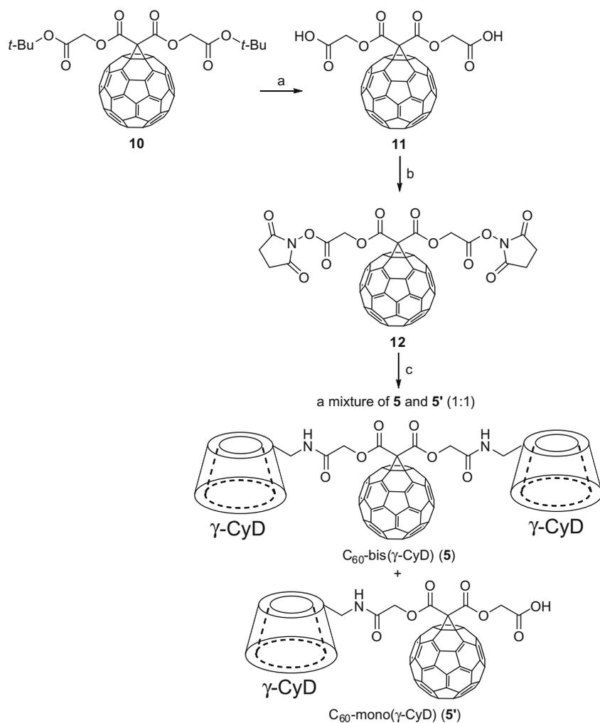
**Scheme 2.** Synthesis of  $C_{60}$ -bis( $\gamma$ -CyD) (**5**) containing  $C_{60}$ -mono( $\gamma$ -CyD) (**5'**). Reagents, conditions, and yields: (a)  $p$ -TsOH, toluene, reflux, 96%; (b) NHS, EDCI, DMF; and (c)  $NH_2$ - $\gamma$ -CyD, DMF, 19% from **11**.
