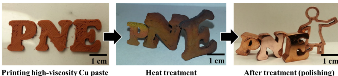
Fig. 8. Complete process for fabrication of 3D metal structures from high-viscosity Cu paste.
