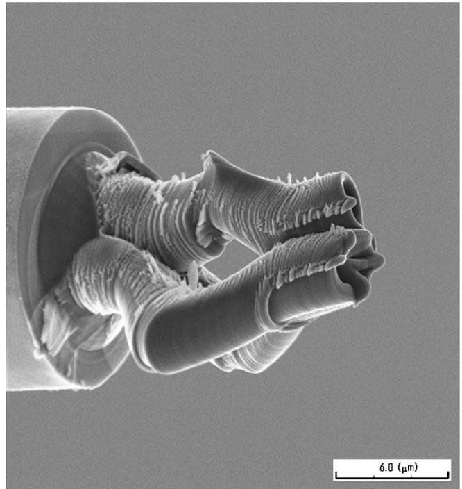
FIG. 1. Bundle of DLC microtubes attached to the edge of a glass capillary. These had an inner diameter of about 2  $\mu\text{m}$ .
