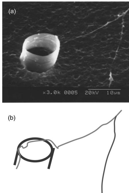
FIG. 8. Axon extension on a microtube attached to a polycarbonate membrane. (a) SEM image of the microtube and the axon. (b) Schematic of SEM image in (a). The axon grew from the upper right of (a) to the microtube, extended along the inner surface of the microtube, and then exited from it.
