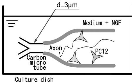
FIG. 4. Schematic of the *in vitro* test using a glass capillary with a bifurcated microtube. The glass capillary and the microtubes were immersed in a culture medium with 50 ng/ml of NGF added. PC12 cells were cultured in the capillary.
