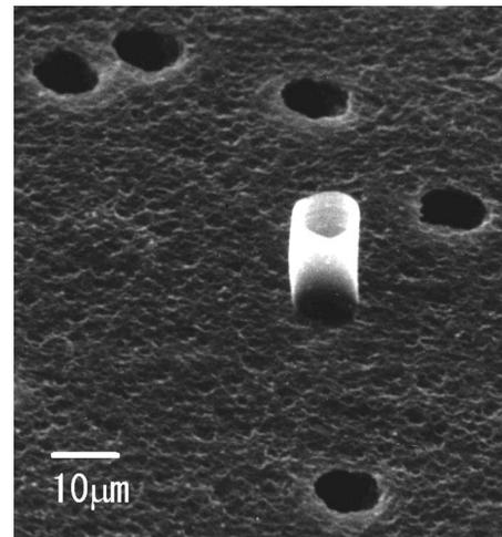
FIG. 3. Carbon microtube on a porous polycarbonate membrane with pore diameter of  $8\ \mu\text{m}$ . The microtube was about  $14\ \mu\text{m}$  in height and  $8\ \mu\text{m}$  in inner diameter as observed by SEM.
