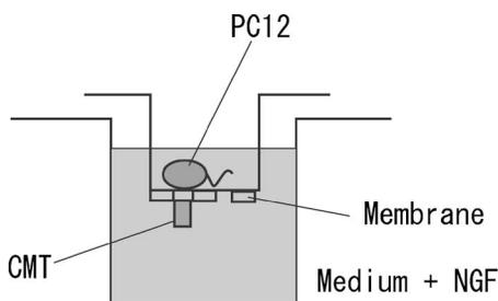
FIG. 5. Schematic of the *in vitro* test using polycarbonate membranes with straight microtubes. The membranes and the microtubes were immersed in a culture medium with 200 ng/ml of NGF added. PC12 cells were cultured on the membranes.
