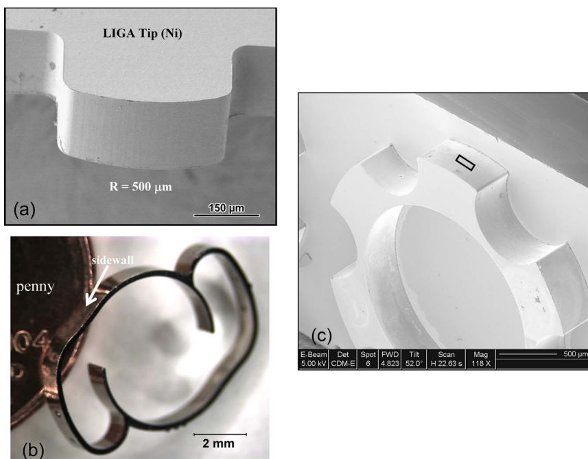
Fig. 3. LIGA-fabricated test structures. (a) Ni friction probe with a 500- \mu\text{m} radius of curvature cylindrical tip. (b) NiMn alloy spring (friction measurement was made on its sidewall). (c) Test structure for characterizing the DLN coating on its sidewall (inset box shows the location at which the FIB section was taken).
