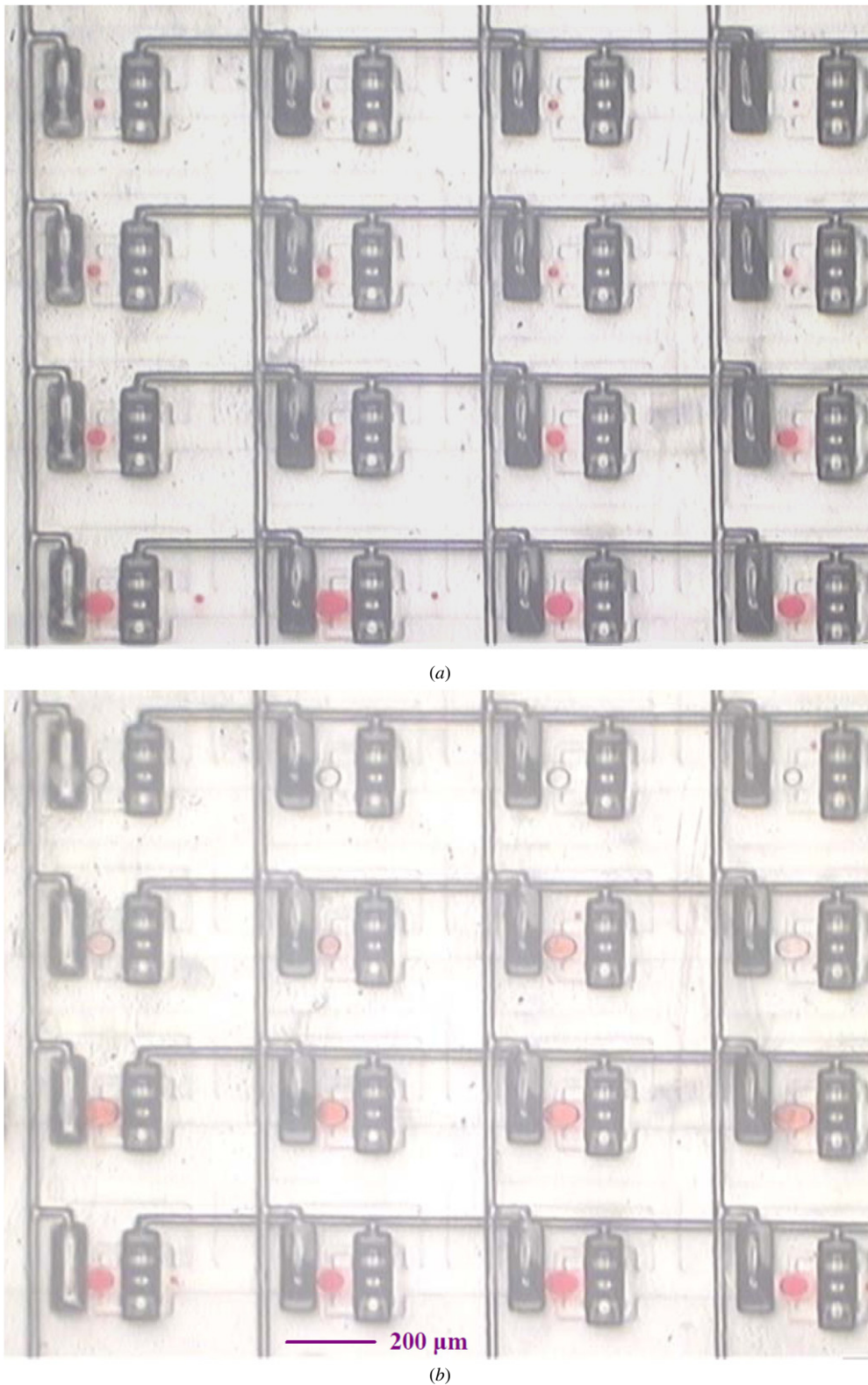
Figure 13. Deposition of 16 droplets with (a) the same concentration but various volumes and (b) various concentrations and volumes in a 4 \times 4 microarray.
