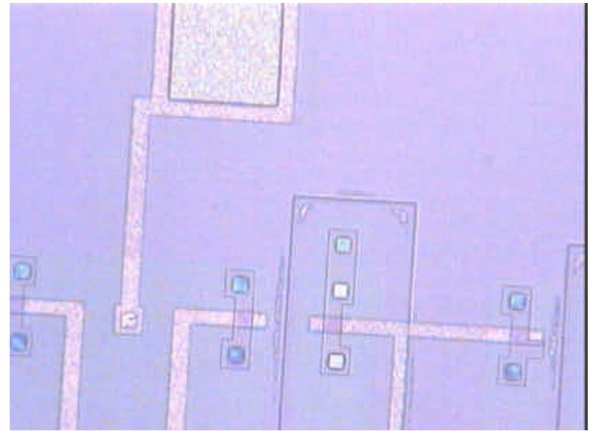
Wet etch has problems with blocking. That is where the BOE can not get into the small contact cut openings. Blocking depends on surface wetting angle. If blocking occurs some contact cuts will etch and clear while others will not etch as illustrated in the pictures above.
