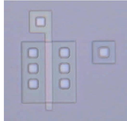
To overcome the blocking problem we raised the boat completely out of the BOE every 15 seconds throughout the entire etch. To be sure to clear all the contacts the etch time was extended to 5 minutes (approximately twice the expected etch time based on etch rates and approximate film thicknesses) This approach gave excellent results for all the various film stacks as shown in the pictures above.
