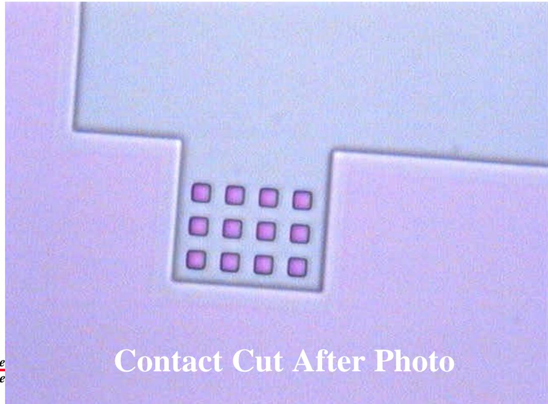
***MAKING SMALL ( $2\mu\text{m} \times 2\mu\text{m}$ ) CONTACT CUT BY WET ETCH***
