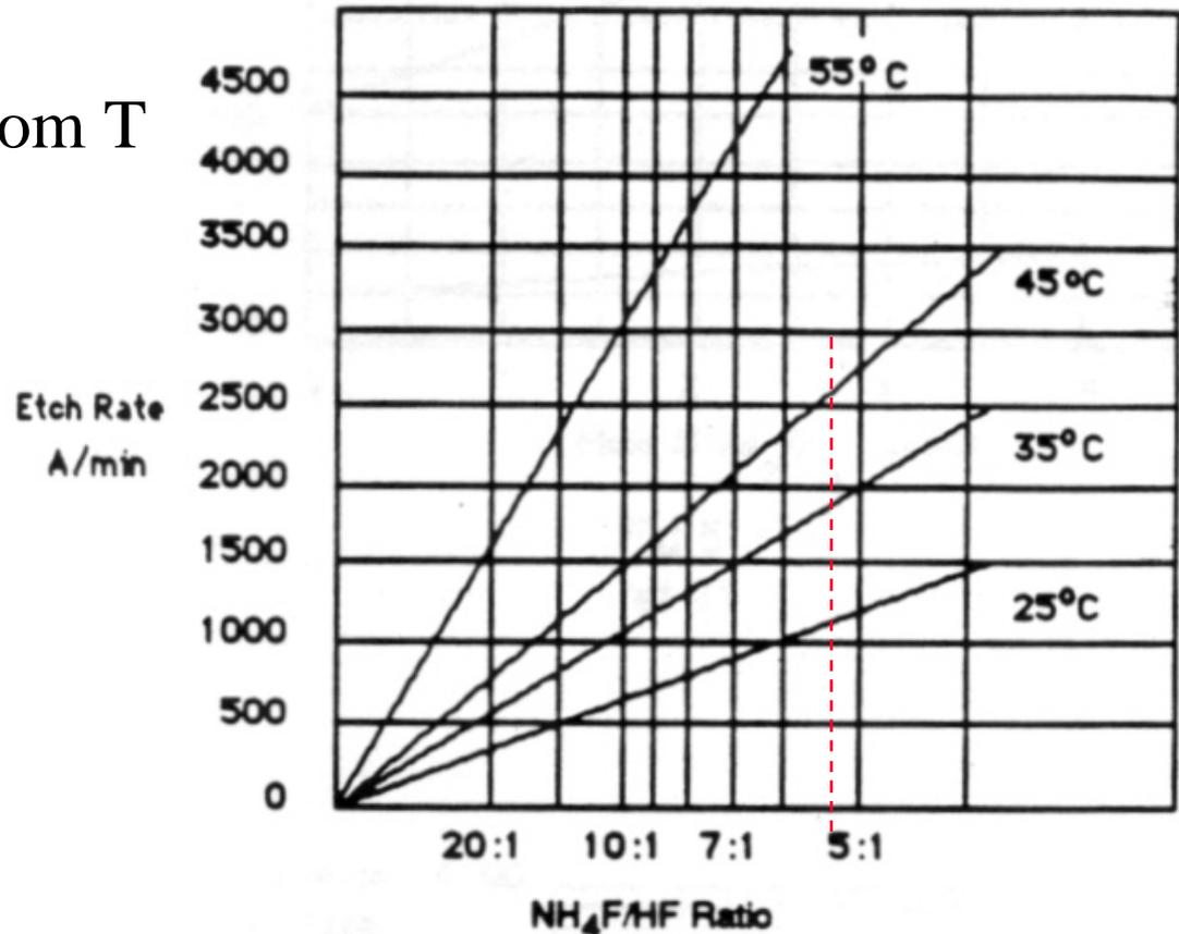
Oxide Etch Rates in Buffered Hydrofluoric Acid
