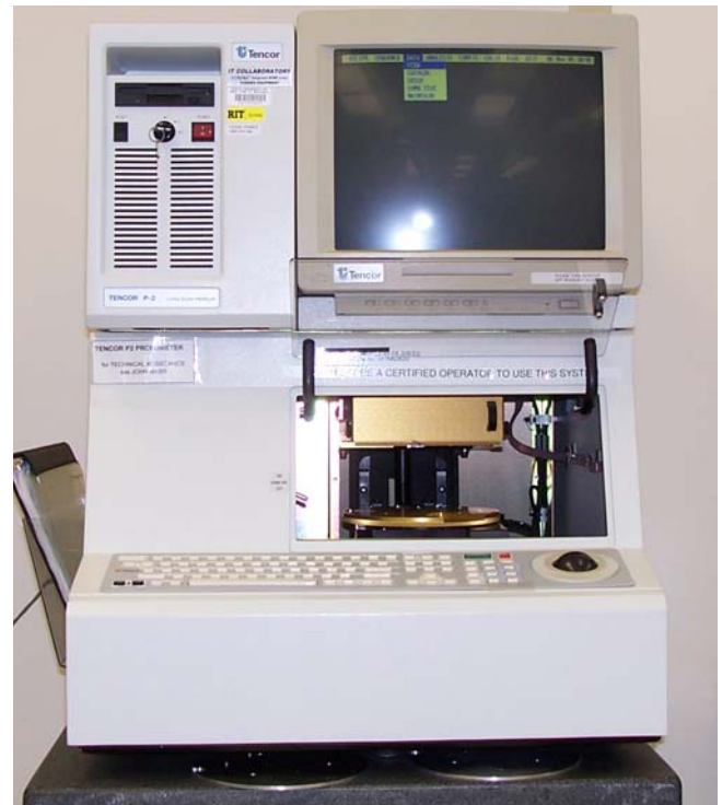
Figure 10. Tencor P2 Long Scan Profilometer. (Left)
