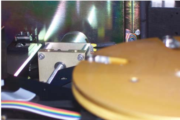
Figure 2. Y Stage driving mechanism. The servo motor can be seen at the back together with the reduction gears and the worm screw.
