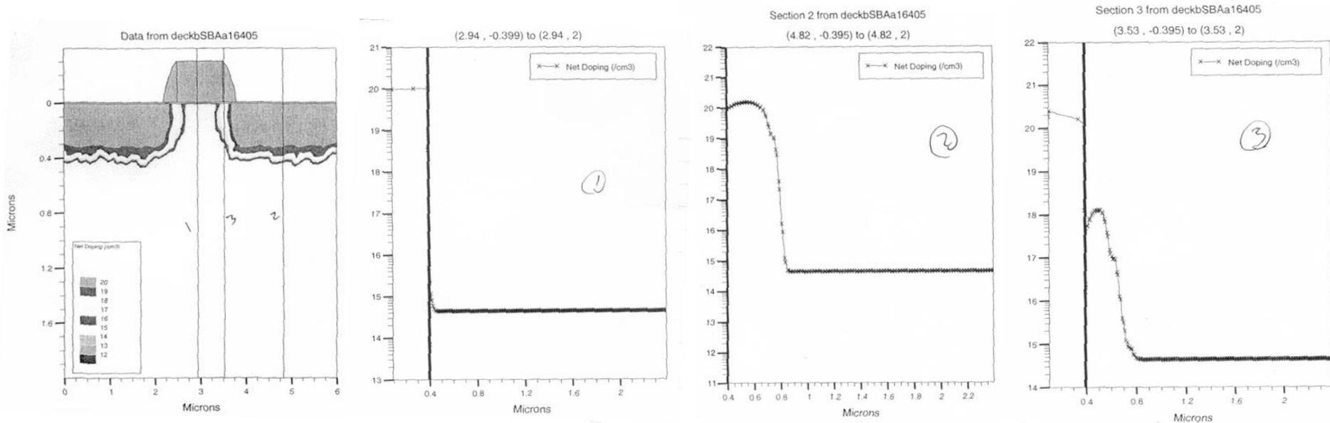
These simulations show that 3000 Å of poly and nitride spacer is enough to block P31 implants from reaching the channel (region 1), the n<sup>+</sup> D/S implant profile is shown in region 2, the LDD n-D/S implant profile is shown in region 3, both after 900 C, 30 min anneal. Note doping  $\sim 1E20$  in D/S and  $\sim 1E18$  in LDD/LDS and  $x_j \sim 0.6 \mu\text{m}$
