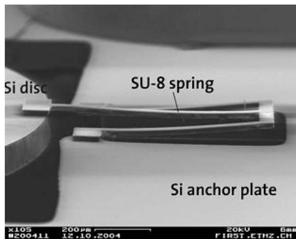
Figure 1. Stress gradient observed in a spring made out of SU-8 [3]
