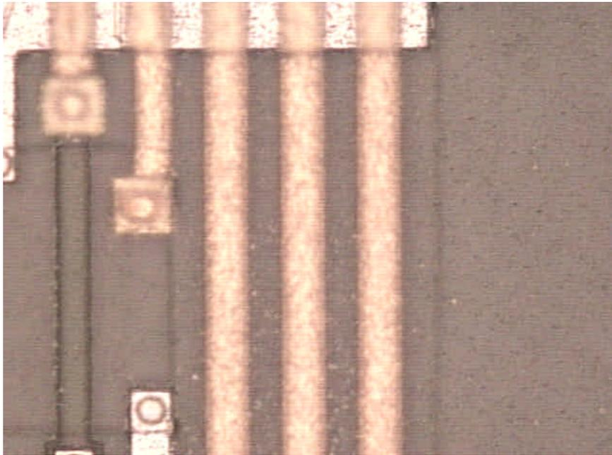
Photoresist on Metal Two
