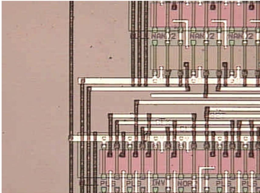
$6\mu\text{m}$  M2 lines with photoresist
