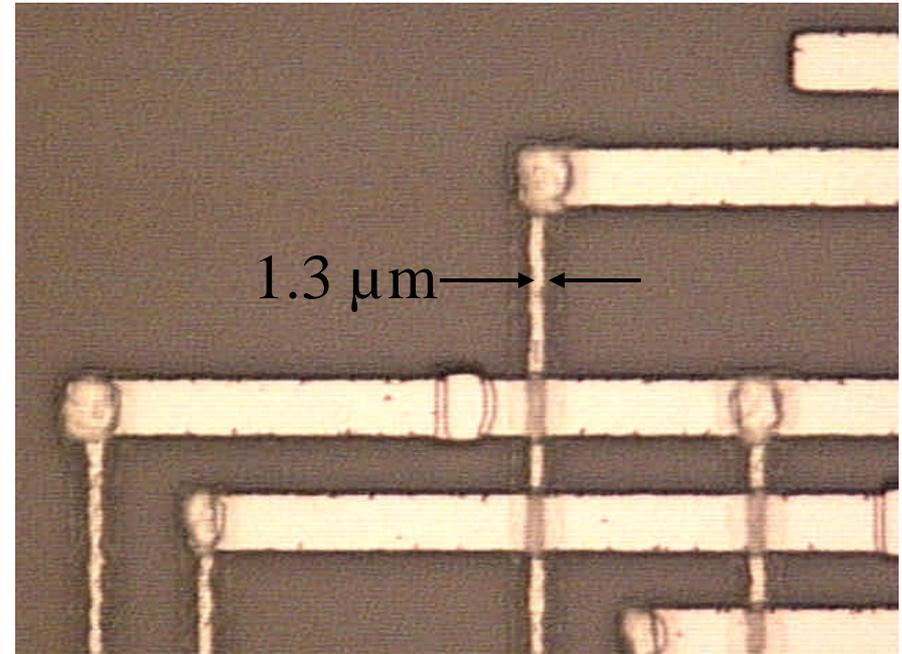
Resist removed show M2 lines are actually  $1.3\mu\text{m}$
