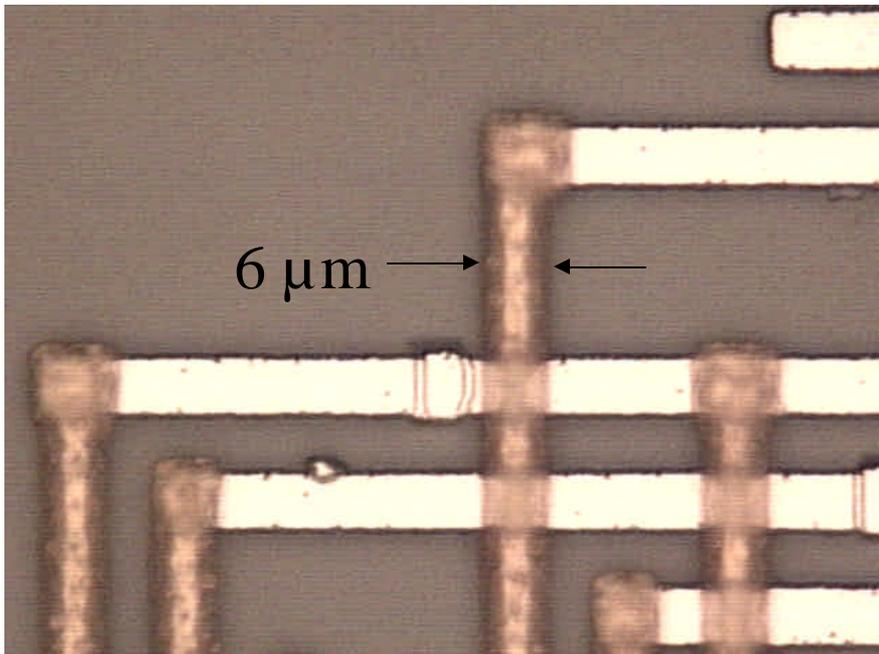
$6\mu\text{m}$  M2 lines with photoresist
