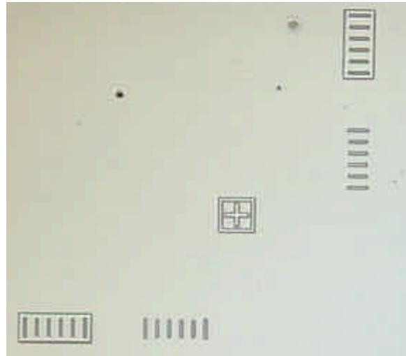
We modified the stepper job F081SUBCMOS\_M2 so that it used the two die with no metal two for alignment and exposed the wafer using the M2 photomask.
