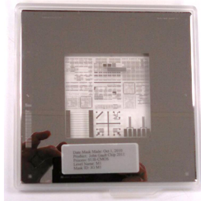
Non Chrome Side As loaded into Reticle Pod, Chrome Down, Reticle Pre- Alignment Stars Sticking out of Pod
