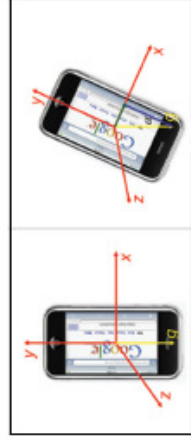
Fig. 3. The orientation of the three independent acceleration-sensors of an iPhone or iPod touch; the sensors measure the acceleration in the direction of the three plotted axes.
