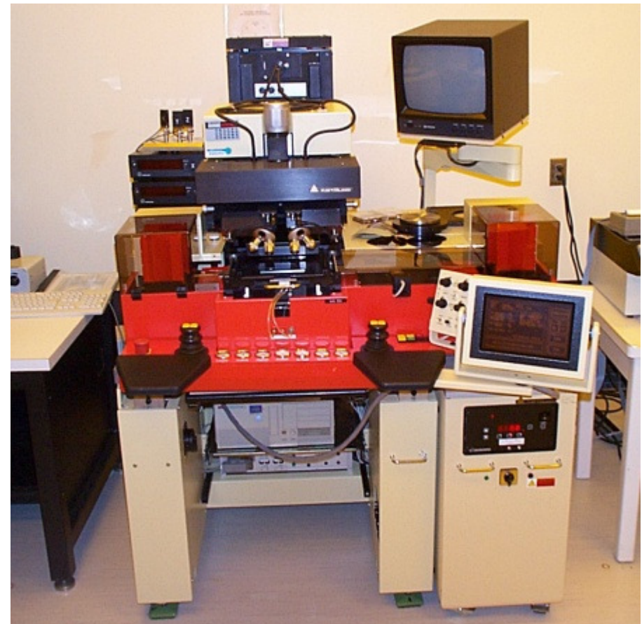
Flood Expose (10 sec = ~ 100mj/cm 2 ) Karl Suss MA150
