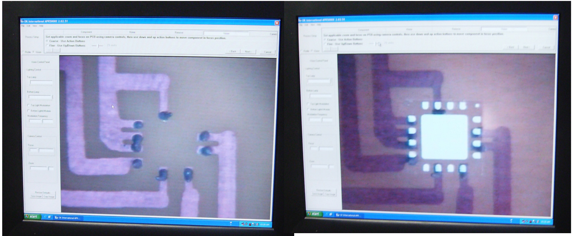
Image of bottom of ADXL325 Superimposed on Copper Traces
