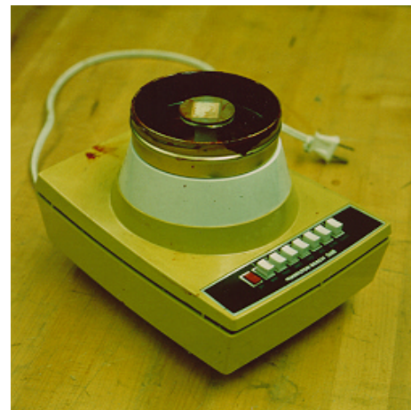
Hamilton Beech Blender Modified for spin coating resist on wafers. Purée gives coating thickness of \sim 1 \mu\text{m}
