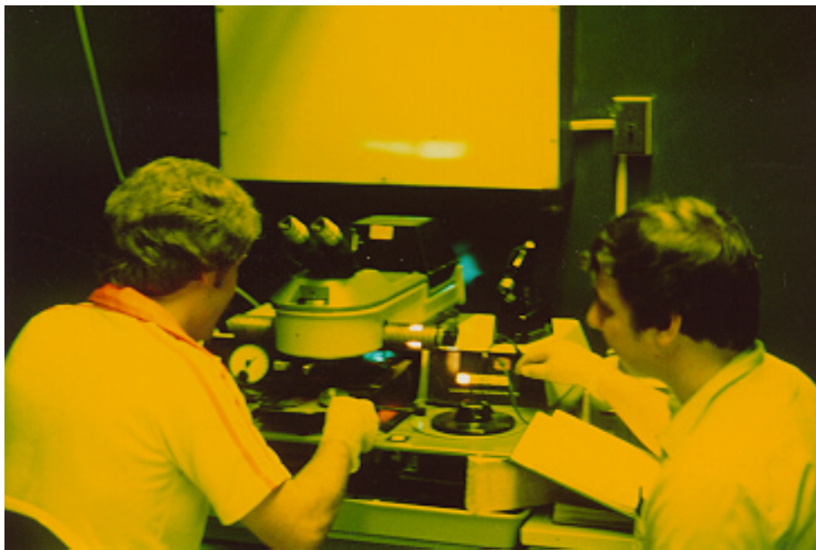
Kasper contact aligner on 2x4 blocks. Notice homemade reduction camera.
