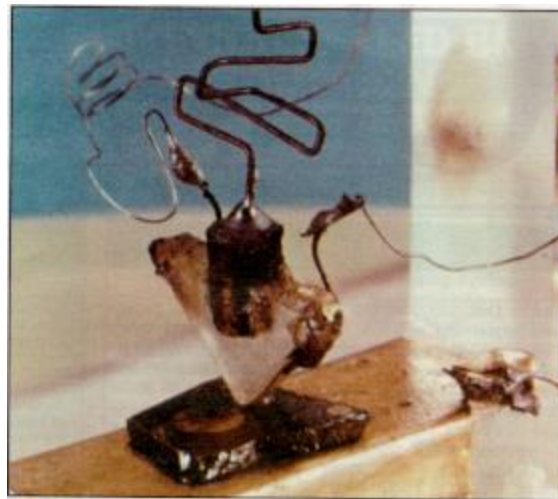
The world's first transistor, built at Bell Labs in December, 1947.
