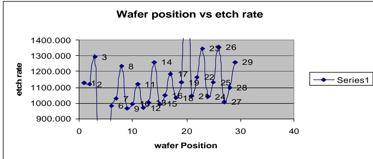
Wafer position Vs Etch rate for wafer #2 on quartz plate
