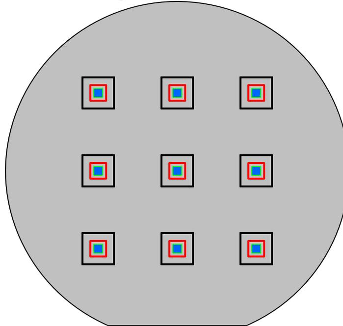
Because higher levels are shifted, need to add shift for TVPA mark locations in each level process file
