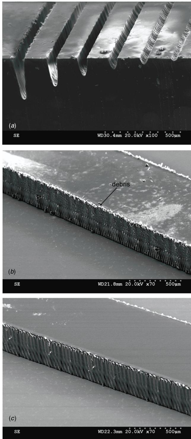
**Figure 6.** (a) At 1000 PPI, the sidewall is neat and clean when cutting the PDMS with a depth smaller than 200 μm and a line width of above 60 μm. (b) Debris appeared on the upper corner when cutting through a 300 μm thick PDMS sheet at 1000 PPI. (c) When reducing the resolution to 600 PPI (~24 pulses per mm), the 300 μm thick PDMS was cut through with little debris.
