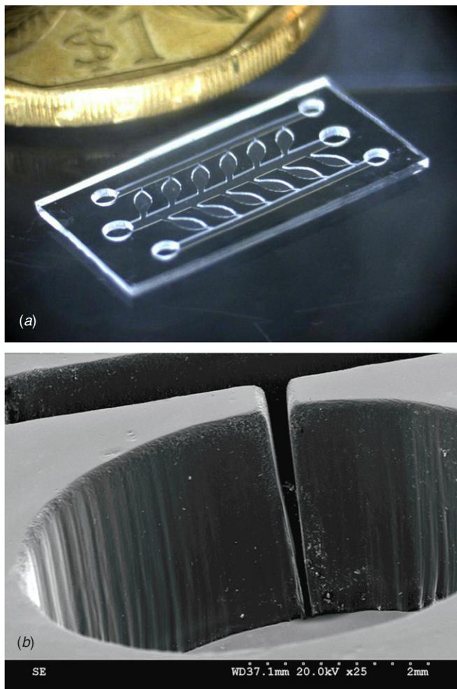
**Figure 2.** (a) A photo of a capillarity-driven microfluidic microreactor array fabricated using the TC&T process. A one Singapore dollar coin is placed beside the chips for size comparison. (b) An SEM image of a high aspect ratio channel and a PDMS chamber with a height of 2.5 mm for cell study.
