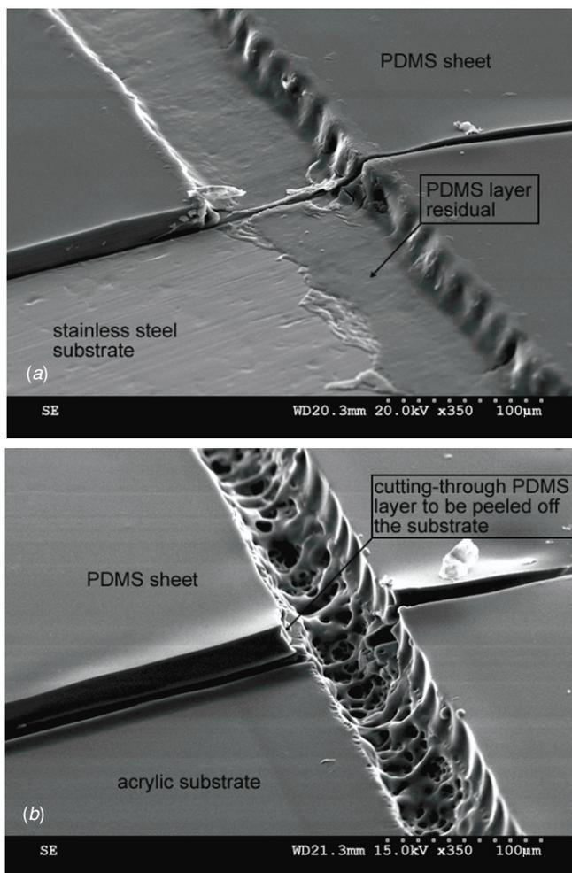
**Figure 3.** Cutting a  $22\ \mu\text{m}$  PDMS sheet on substrates made of different materials. The PDMS layer on the bottom left was knife cut and removed. (a) On a stainless steel substrate, the PDMS layer cannot be cut through totally even with large laser power, leaving a thin layer of the PDMS residual on the substrate. (b) On an acrylic substrate, the laser can cut through the PDMS layer, leaving a groove over the acrylic surface.
