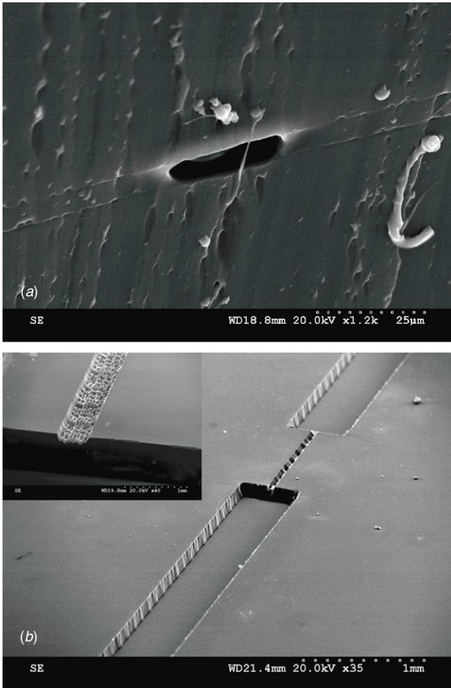
**Figure 5.** (a) Cross-sectional view of a PDMS microchannel with a height of  $7\ \mu\text{m}$  which is controllable by forming a PDMS layer of the same thickness for laser through-cutting. (b) Channels with different widths and depths formed by a combined use of the through-cutting and the blind-engraving techniques. The wide channel has a smoother bottom when compared with the channel bottom formed by the raster scan (the inset).
