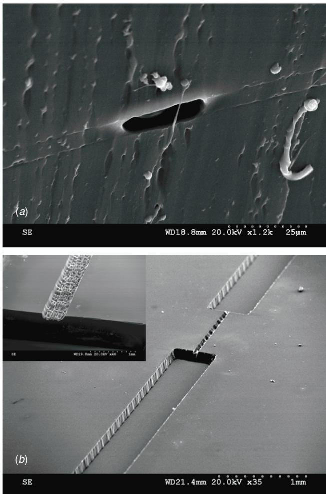
**Figure 5.** (a) Cross-sectional view of a PDMS microchannel with a height of 7 μm which is controllable by forming a PDMS layer of the same thickness for laser through-cutting. (b) Channels with different widths and depths formed by a combined use of the through-cutting and the blind-engraving techniques. The wide channel has a smoother bottom when compared with the channel bottom formed by the raster scan (the inset).
