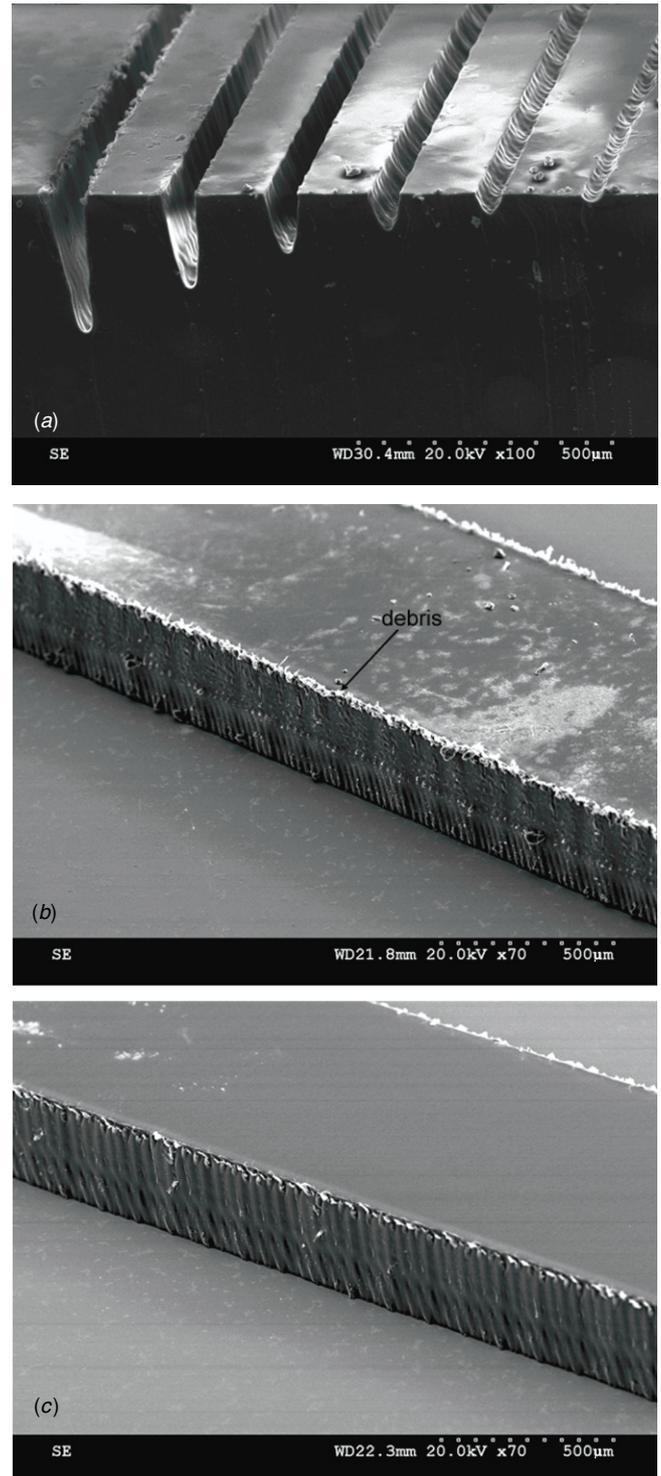
**Figure 6.** (a) At 1000 PPI, the sidewall is neat and clean when cutting the PDMS with a depth smaller than  $200\ \mu\text{m}$  and a line width of above  $60\ \mu\text{m}$ . (b) Debris appeared on the upper corner when cutting through a  $300\ \mu\text{m}$  thick PDMS sheet at 1000 PPI. (c) When reducing the resolution to 600 PPI ( $\sim 24$  pulses per mm), the  $300\ \mu\text{m}$  thick PDMS was cut through with little debris.
