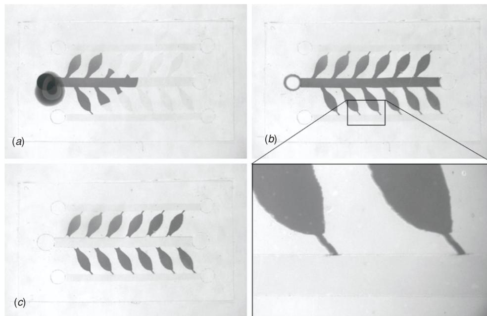
**Figure 7.** Microfluidic test using the PDMS chip fabricated by a pulsed CO<sub>2</sub> laser. (a) Liquid loading process. (b) Liquid retained in the leaf reactors without leaking to the air venting channels due to confinement of the narrow openings of the passive valves. (c) Liquid remained inside the leaf reactors after removing the liquid in the stem channel by an absorbent.
