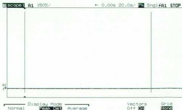
Fig. 2. A display of a long time window in peak detection mode, showing a 100-nanosecond event at a time-per-division setting of 20 seconds per division. To detect this event without peak detection would require at least a 10-MSa/s sample rate and a memory depth of two billion samples.
