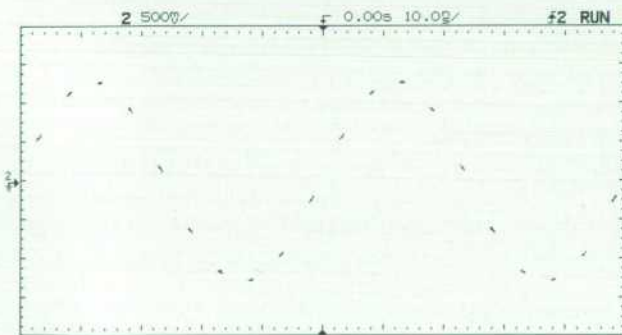
Fig. 2. The result of applying a sine wave with a frequency equal to precisely 1/10 the sample clock frequency to a random repetitive sampling digital oscilloscope. All sets of samples accumulate around the same locations.
