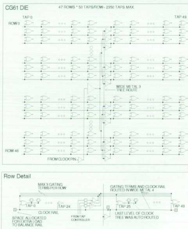
Fig. 5. Clock distribution tree.
