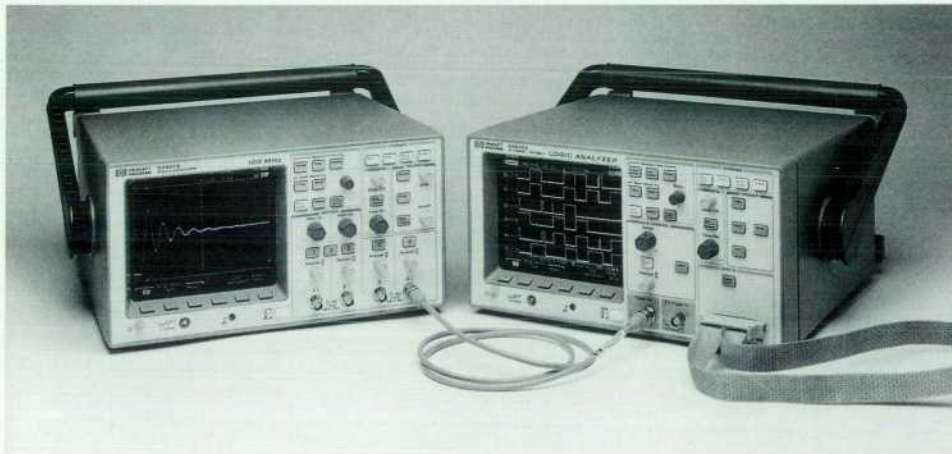
Fig. 1. The HP 54620 logic timing analyzer can trigger on a complex set of digital signals and provide its trigger signal to an oscilloscope to display a resulting analog signal.
