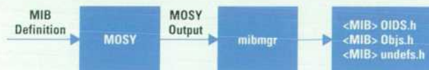
Fig. 8. The process of automatically generating of C++ header files for network applications using SNMPGen.
