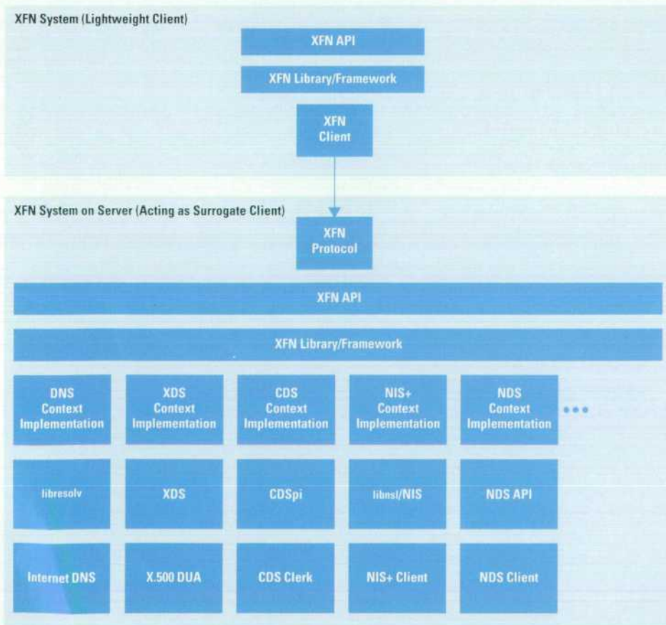
Fig. 4. Lightweight XFN client configuration with surrogate client on server.
