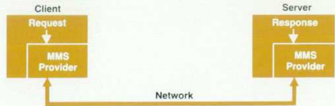
Fig. 7. Process of communication in MMS.
