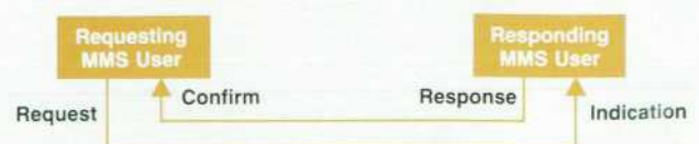
Fig. 2. MMS services are either confirmed or unconfirmed. The response shown is omitted for unconfirmed services.
