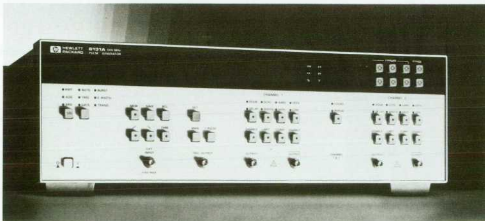
Fig. 1. HP 8131A 500-MHz pulse generator with fixed 200-ps rise and fall times (optional two-channel version).
