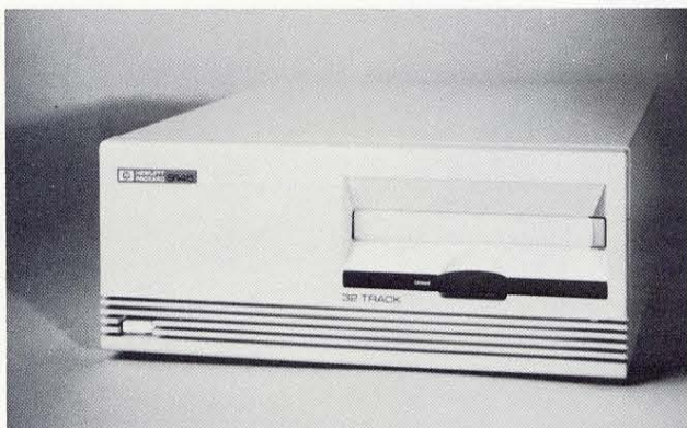
Fig. 1. The HP 9145A 1/4-Inch Tape Drive provides a storage capacity of 133 Mbytes per cartridge and a data transfer rate of 4 Mbytes per minute for backing up disc memory in entry level and midrange computer systems.
