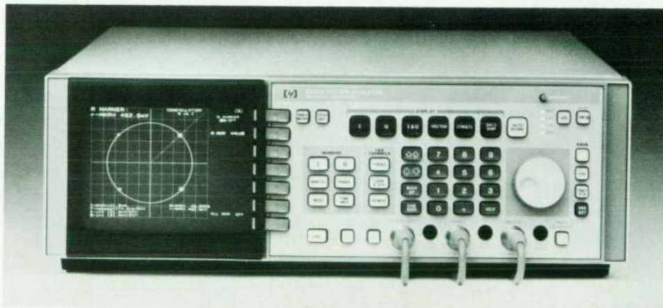
Fig. 1. The HP 8980A Vector Analyzer is a 350-MHz two-channel X-Y sampling oscilloscope designed to characterize the in-phase and quadrature components of modern communications and radar system signals.
