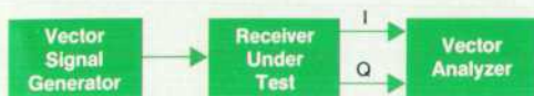
Fig. 2. Recommended test setup for obtaining the correct constellation diagram of a 16QAM radio.
