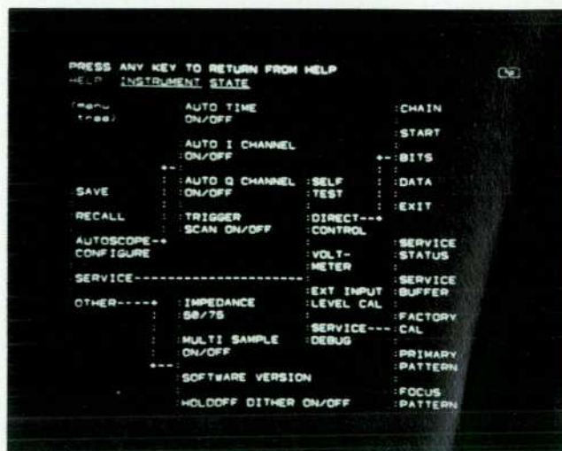
Fig. 7. Menu tree invoked by INSTR STA (instrument state) key.
