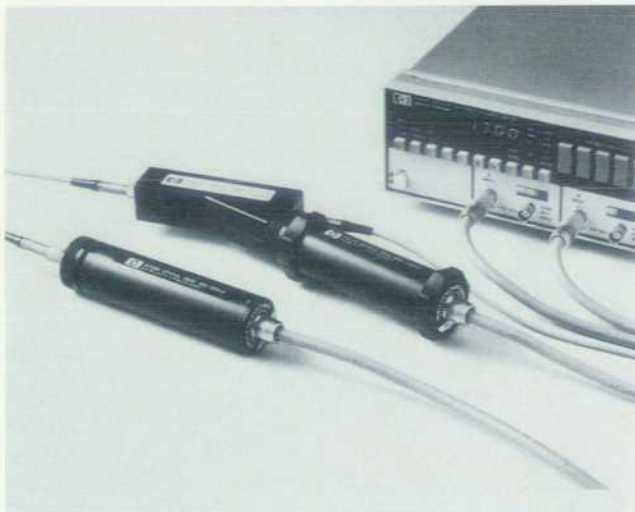
Fig. 1. The programmable, two-channel HP 8152A Optical Average Power Meter has accuracy as high as \pm 0.15 dB for both absolute and relative power measurements. It operates with the HP 81520A Optical Head from 450 to 950 nm and with the HP 81521B Optical Head from 850 to 1700 nm.
