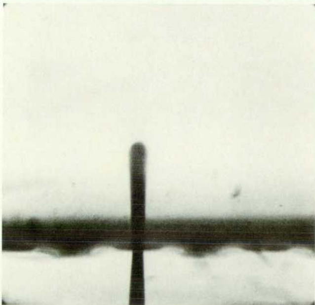
Fig. 8. Photomicrograph of the ejection of an ink droplet 20 \mu s after the application of the electrical pulse to the heater.
