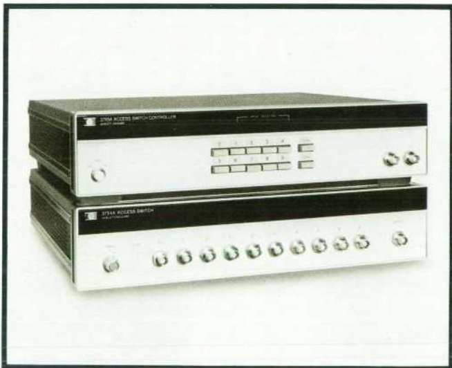
Fig. 1. Model 3754A Access Switch (lower unit) connects any one of ten RF inputs to a single output under control of the Model 3755A Access Switch Controller (upper unit). Inputs can be selected manually by way of the Controller's front panel pushbuttons or under automatic control by way of the HP interface bus. LED indicators in the dark panel above the Access Switch inputs light up to show which input is connected to the output.
