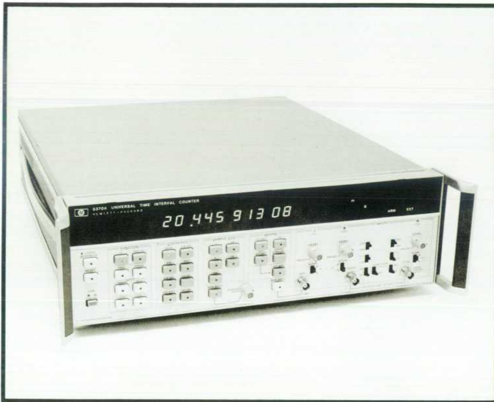
Fig. 1. Model 5370A Universal Time Interval Counter measures time intervals from -10 to +10 seconds with 20-ps resolution in single-shot measurements. It can compute the mean, standard deviation, maximum, and minimum of repetitive time intervals. It measures frequency to 100 MHz, giving 11-digit resolution in one second. HP-IB interface and remote programmability are standard features.
