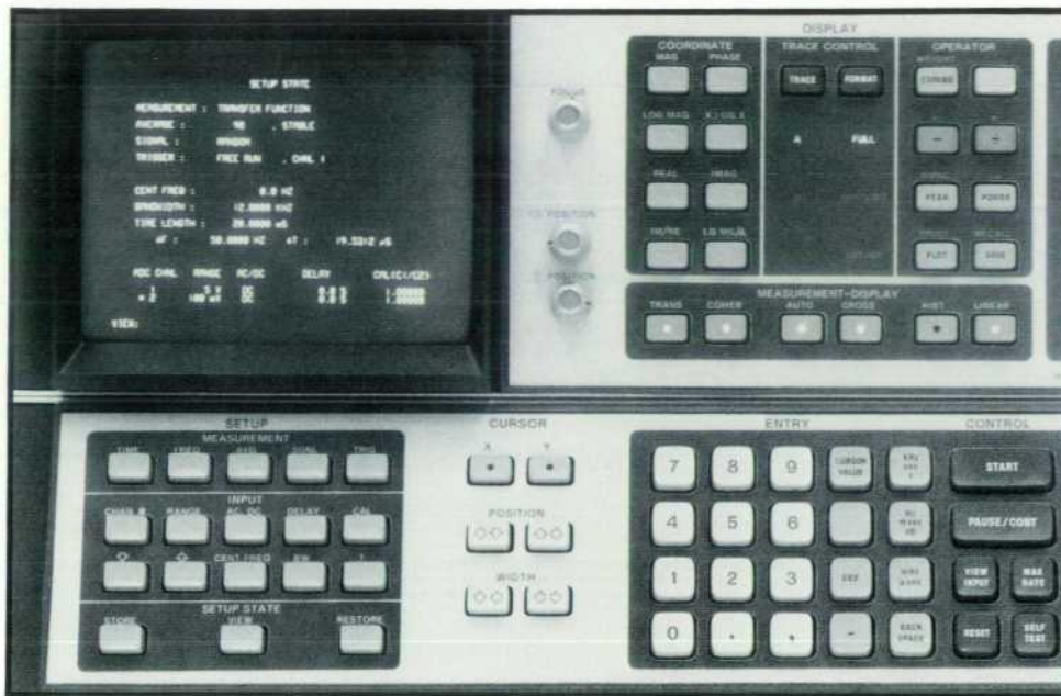
Fig. 3. CRT display extends the front panel, helping to make the new analyzer easy to use for both the novice and the experienced operator. For example, pushing the VIEW key causes the instrument's status to be displayed. Other keys display lists of choices from which the user can select measurement parameters.
