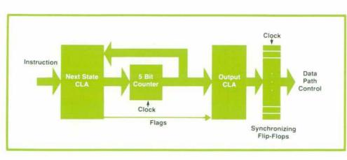
Fig. 8. MC<sup>2</sup> control section block diagram. Custom logic arrays (CLAs) are like programmable logic arrays (PLAs, a form of readonly memory) but do not have a full output matrix. The CLAs are controlled by a five-bit counter.
