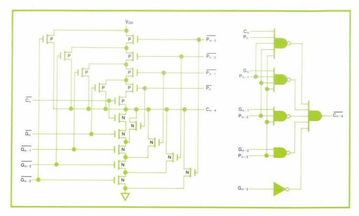
Fig. 7. The ALU uses functional gating to save area and generate a 16-bit carry in 35 ns; only half the number of transistors are needed as for a conventional gate realization. Four-bit look-ahead is used in generating the 16-bit carry. There are four carry look-ahead circuits like the one shown here. The ripple method is used within each four-bit block; the combination of methods also helps save area.
