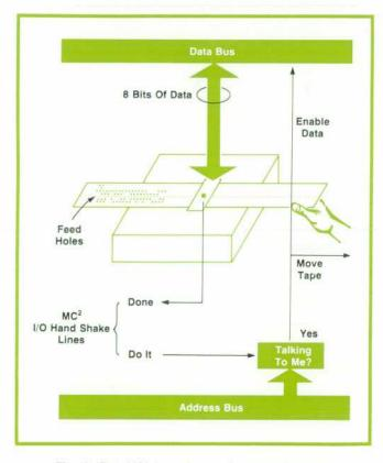
Fig. 2. The MC<sup>2</sup> is optimized for controller applications, and treats I/O devices as banks of registers. This simple paper tape reader interface takes advantage of the processor's static and asynchronous properties and direct I/O manipulation.
