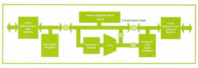
Fig. 5. MC<sup>2</sup> data path block diagram. External registers used for I/O operations are treated in the same way as the internal registers. This allows flexibility in manipulating data while keeping the length of instructions to a minimum.
