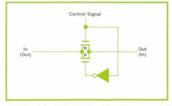
**Fig. 6.** Logic blocks in the data path are connected to the main bus by full complementary transmission gates. These gates are fast (<1.5 ns delay), small (540  $\mu$ m<sup>2</sup>), and bidirectional, thereby simplifying complex logic implementation.
