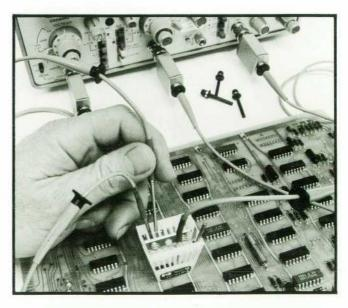
Fig. 5. Miniature probe with insulating sleeve removed is held in place on an IC lead by the optional IC clip. The bare ground-reference pin, shown here in the right-hand corner of the clip, can be inserted at any lead position. It grounds reference planes within the clip that in turn contact the barrel of the probe(s). Risetimes as short as 1.3 ns are preserved by this arrangement (Fig. 6).
