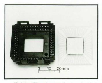
**Fig. 9.** The MC<sup>2</sup> is packaged on a 48-pad ceramic substrate. A special low-insertion-force socket is used.
