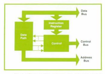
Fig. 4. MC<sup>2</sup> basic block diagram. The data path consists of four blocks of logic that may be connected to a common internal bus or operated independently. See Fig. 5.
