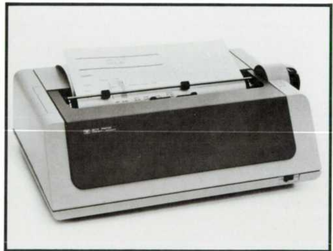
Fig. 1. Model 9871A Printer is a page-width impact printer for use with all HP 9800-Series Calculators. It prints up to 132 columns at 10 characters per inch. Printing speed is 30 characters per second.
