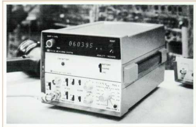
Fig. 10. Battery pack fits between mainframe and snap-on module. It has handles and a detachable shoulder strap.
