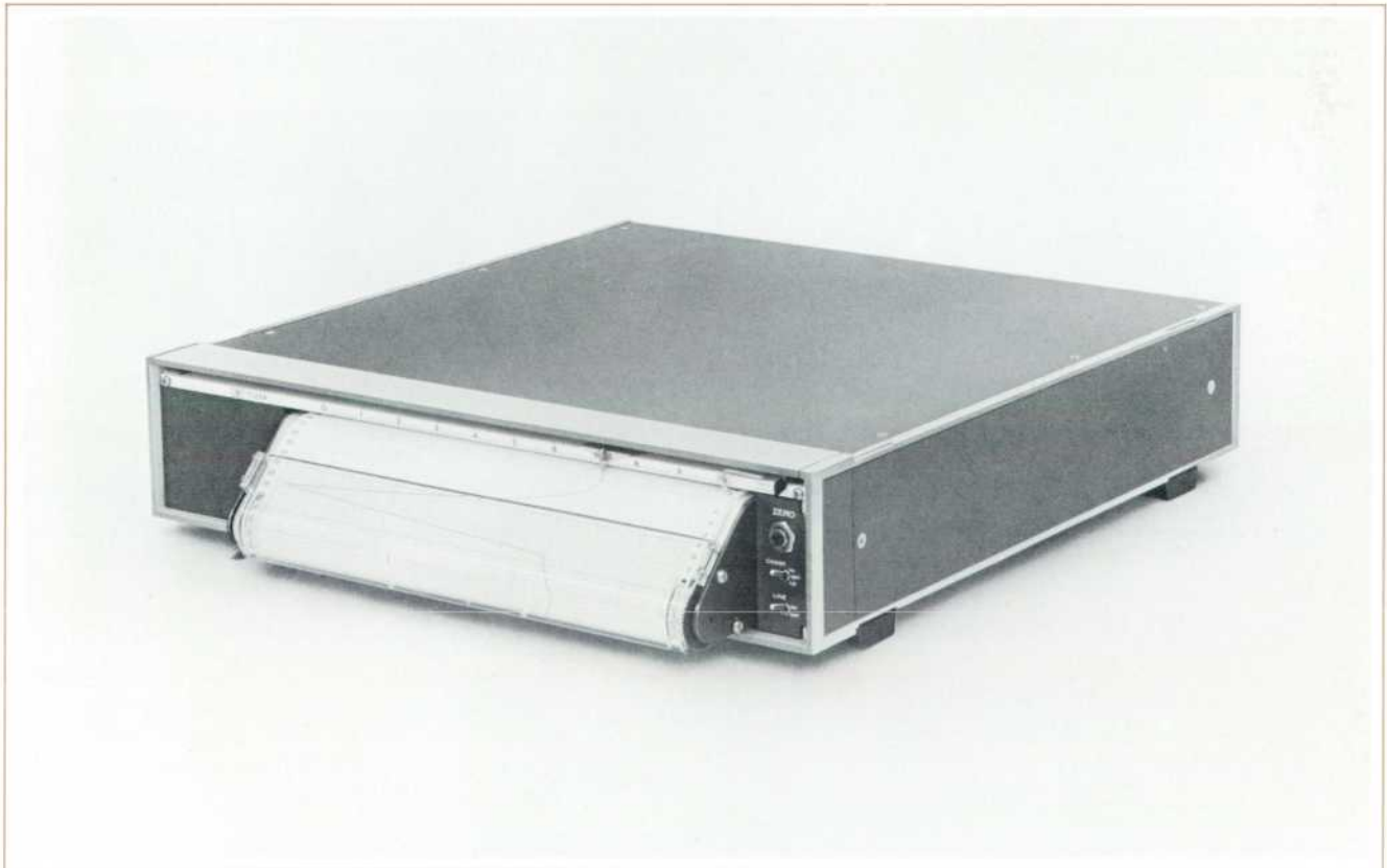
Fig. 1. This new Hewlett-Packard Model 7123A/B Strip Chart Recorder has been developed specifically for dedicated applications. The linear servo motor has only one moving part and has high reliability.
