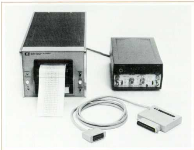
Fig. 9. Serial-to-parallel converter at end of accessory cable converts BCD output of 5300A mainframe to parallel form required by many printers.
