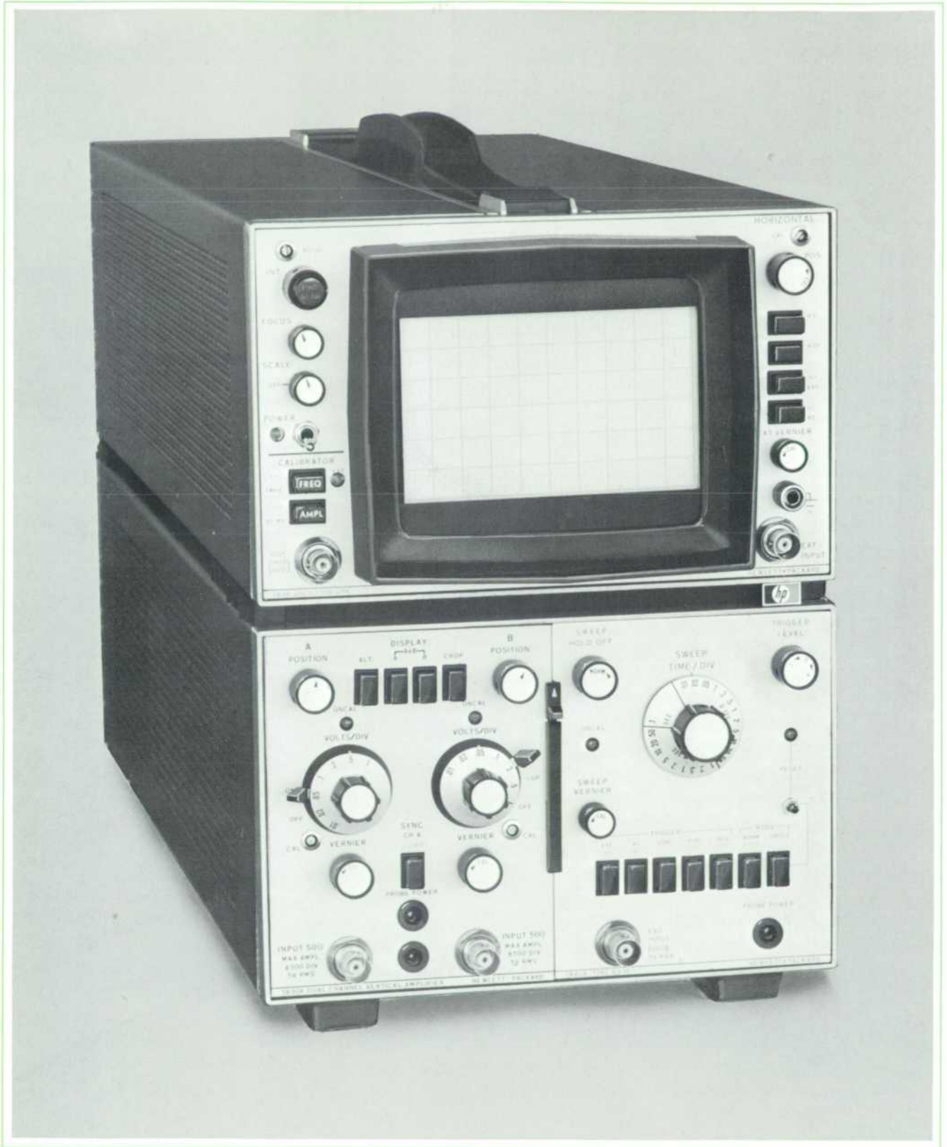
Fig. 1. New Model 183A Oscilloscope mainframe with 1830A and 1840A plug-ins has dual-channel, 250 MHz, 10 mV/cm response and sweep times to 1 ns/cm (with mainframe \times 10 magnifier). Scope has 4 ns/cm photographic writing rate.
