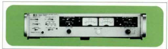
Fig. 3. Model 8717A Transistor Bias Supply has slide switches for rapid selection of bias conditions. The transistor being biased is an integral part of a feedback system in the supply which maintains the accuracy and stability of the bias conditions.
