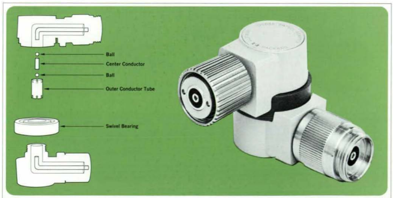
Fig. 10. Flexible cables couldn't be used in the network analyzer system because they have high reflection coefficients and because the phases and amplitudes of signals change when the cables are moved. To replace cables, this swivel adapter was developed, along with a rotary air line which uses the same double-ball-joint construction. Combinations of adapters and rotary lines can make the same connections that flexible cables can, yet have the accuracy of rigid coaxial lines.
