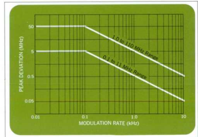
Fig. 5. Typical measured curves for 1% distortion of external FM. Generator/sweeper introduces less than 1% distortion as long as FM rate and deviation are below solid line (except that for peak deviations below bottom of graph, distortion begins to increase because of noise).
