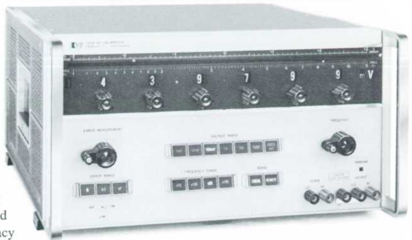
Fig. 2. This new Model 745A AC Calibrator is a precision signal generator designed to provide ac voltages to \pm 0.02\% accuracy at midband. Frequency range is continuously adjustable from 10 Hz to 110 kHz. The percent error scale enables direct error measurement without the necessity for calculation. Voltage, frequency, error ranges and frequency vernier may be programmed.
