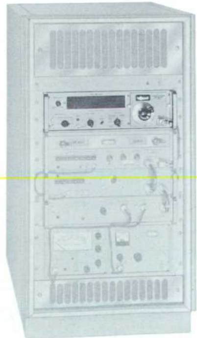
Fig. 6. Hewlett-Packard 0.3-3 Gc Frequency Converter and 50 Mc Counter (upper unit) as used in Boonton Radio's 8925A Test Set which calibrates and tests DME (distance measuring equipment) and ATC (air-traffic control) airborne transponders. Counter and converter monitor signal generator output, which is modulated by external pulses to simulate DME and ATC pulses for transponder receiver, throughout 950-1250 Mc range.
