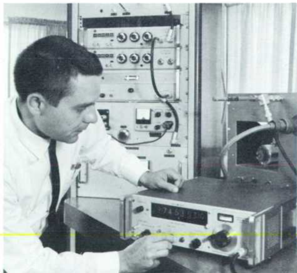
Fig. 1. New -hp- 300 to 3000 Mc Converter being used with -hp- 5245L Counter at backscatter range facility of Micronetics, Inc., San Diego, Calif. Converter and counter are used in precisely establishing UHF, L-band, and S-band frequencies used in making radar cross-section measurements. Here, Warren T. Fey, techniques engineering manager, checks frequency of one of Micronetics' range transmitters.
