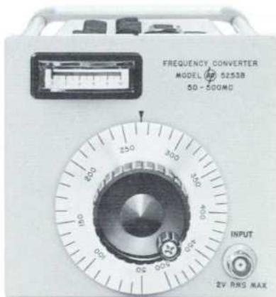
Fig. 8. Companion Frequency converter, -hp- Model 5253B, measures from 50 to 500 Mc, completes frequency coverage. Counter and two frequency converters thus span frequency measurement range of dc to 3000 Mc. This plug-in is similar in basic concept to the 0.3-3 Gc converter.
