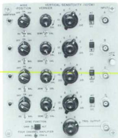
Fig. 6. Each channel of -hp- Model 1754A Four-Channel Plug-in Amplifier has independent controls. Mode Switch has "Off" position which removes any unneeded channel from CRT display.
