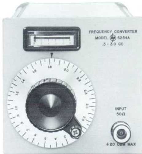
Fig. 7. Hewlett-Packard Model 5254A Frequency Converter enables -hp- 50 Mc counter to make frequency measurements within 300 to 3000 Mc range. Tuning dial, calibrated at multiples of 50 Mc, selects harmonic of 50 Mc signal to be subtracted from input signal. Meter shows when converter is tuned to harmonic that is within 53 Mc of input.
