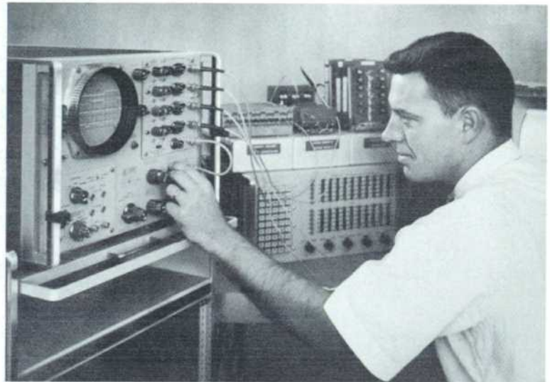
Fig. 1. New Plug-in for -hp- Model 175A Oscilloscope enables simultaneous viewing of up to four waveforms by means of four identical 40-Mc channels. Front panel switch selects waveform from any channel to serve as sweep trigger for all traces, giving extra convenience in examining time-related waveforms.
