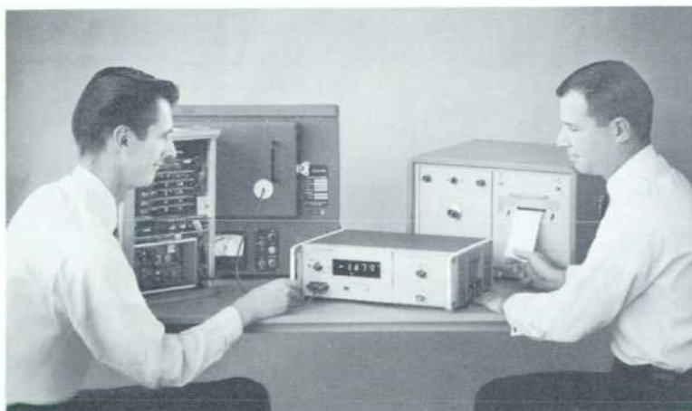
Fig. 1. Front panel plug-ins adapt Model 3440A Digital Voltmeter to manual or automatic ranging for bench use or remote ranging for systems use. Unit shown in center foreground is working with -hp- Model 562A Printer to record voltage/temperature characteristics of circuit operating in environmental chamber. New voltmeter measures dc voltages to an accuracy better than 0.05% of reading \pm 1 count.
