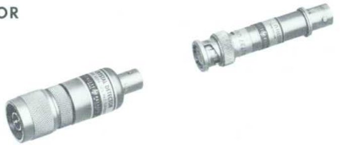
Fig. 1. New -hp- Model 423A Crystal Detector has so constant a frequency response over the 1240:1 range from 10 megacycles to 12.4 gigacycles that any two of the Detectors constitute a well-matched pair. Illustration also shows optional video load which is selected for optimum Detector square-law response.
