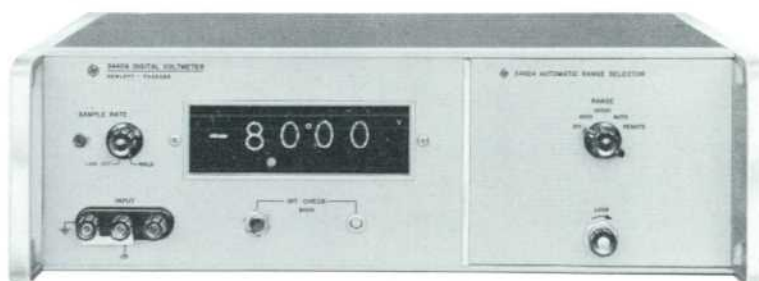
Fig. 4. Model 3440A Digital Voltmeter uses closely-spaced rectangular Nixie® tubes to achieve numerical display with readable span. Readout system has display storage which retains previous reading while new measurement cycle is in process, insuring steady, flickerless display that changes only when input voltage changes. Front panel calibrate button furnishes quick operational check of voltmeter accuracy.
