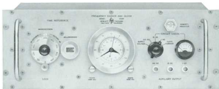
Fig. 1. -hp- Model 113AR Frequency Divider and Clock increases the precision with which local frequencies can be compared with broadcast standard.
