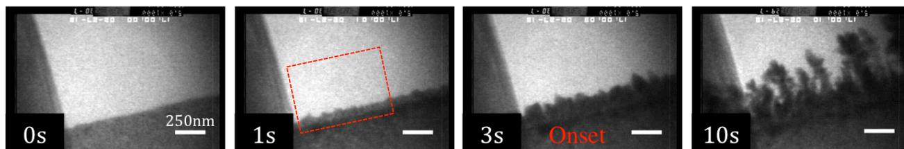
**Figure 1.** Instantaneous micrographs of the growth interface for Cu deposition from acidified  $\text{CuSO}_4$  with an experimentally measured current density of  $1500 \text{ A/m}^2$  for galvanostatic conditions with  $400 \text{ nA}$  total applied depositional current. Red outline represents analyzed region.
