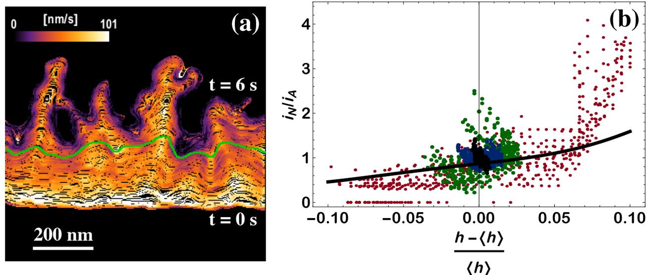
**Figure 2.** (a) “Heat Map” of normal growth speed (akin to point-wise current density) with the measured transition time overlaid in green. (b) Current density normalized by average current density as a function of deviation from the mean height. Data extracted from the growth of **Figure 1** at  $t = 0.0$  (black),  $2.0$  (blue),  $3.0$  (green),  $3.8$  (red) s. Solid line represents sinusoidal solution from [6].
