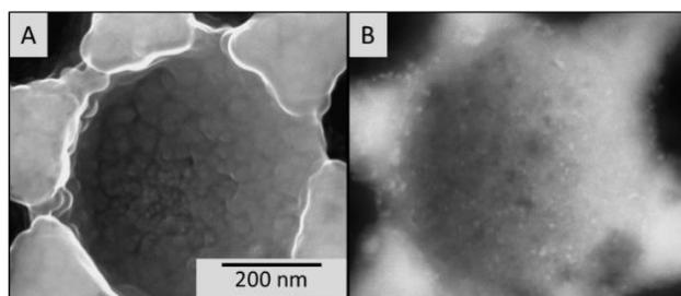
**Figure 1.** Scanning electron micrographs of Pd NPs decorated onto the surfaces of Ni nano-bowls as imaged under the field-free mode by: (A) an Everhart-Thornley electron detector; and (B) a concentric backscattered electron detector.
