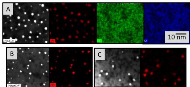
**Figure 2.** (A) Transmission electron microscopy high angle annular dark field (HAADF) image and Pt, Ti, and O EDS maps of  $\text{TiO}_2$  supported Pt NPs. HAADF image and Pt EDS maps of samples prepared from (B) 60% and (C) 90% less Pt NPs.
