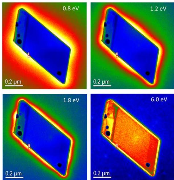
**Figure 1.** EFTEM images which shows of localized plasmons excitation in a Bi<sub>2</sub>Se<sub>3</sub> nanoplates.
