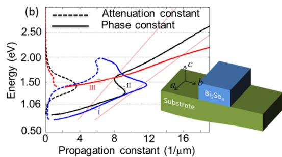
**Figure 2.** Propagation constant of plasmon polaritons propagating in a channel waveguide made of Bi<sub>2</sub>Se<sub>3</sub>.
