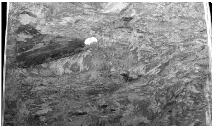
Figure 3. Ferritic steel from a nuclear pressure vessel sectioned with FEI Helios plasma FIB DualBeam at 59 nA Plasma current and 30kV. The slice thickness is 100 nm and the sections face is 100 \times 96 \mu\text{m}^2 with the pixel size of 29 nm. Combined PFIB milling and SEM imaging of a single slice is about 8 minutes. FEGSEM imaging at 2kV, 0.80nA, TLD detector and field-free mode.
