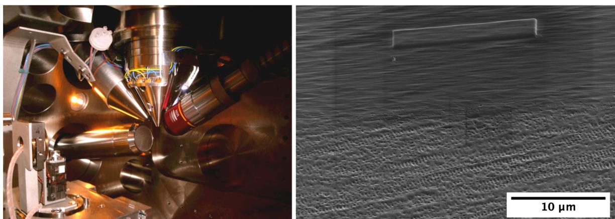
**Figure 1.** (left) The TriBeam tomography FIB-SEM vacuum chamber interior. (right) A silicon sample that was femtosecond laser ablated and then  $\text{Ga}^+$  ion milled at glancing angle (top half of micrograph). The location of a TEM lamella liftout is visible as a raised platinum deposited area.
