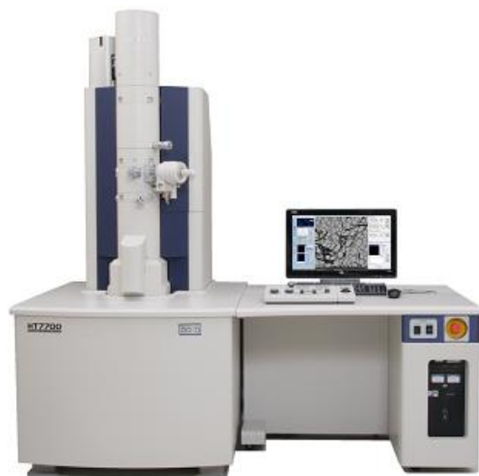
Figure 1. External view of 40-120 kV high resolution analytical TEM.
