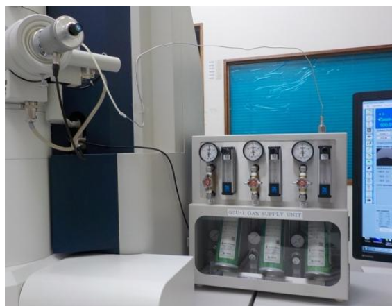
Figure 2. External view of the gas supply system installed on the operation board of a TEM.
