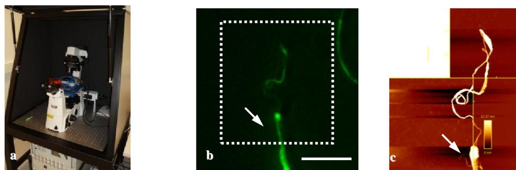
**Figure 2.** Bio-science AFM images: (a) JPK NanoWizard II (b) fluorescent image and (c) combined AFM image on the same area: the plasmid-DNA is only visible by AFM as indicated by white arrows. Scale bar is 20  $\mu$ m.
