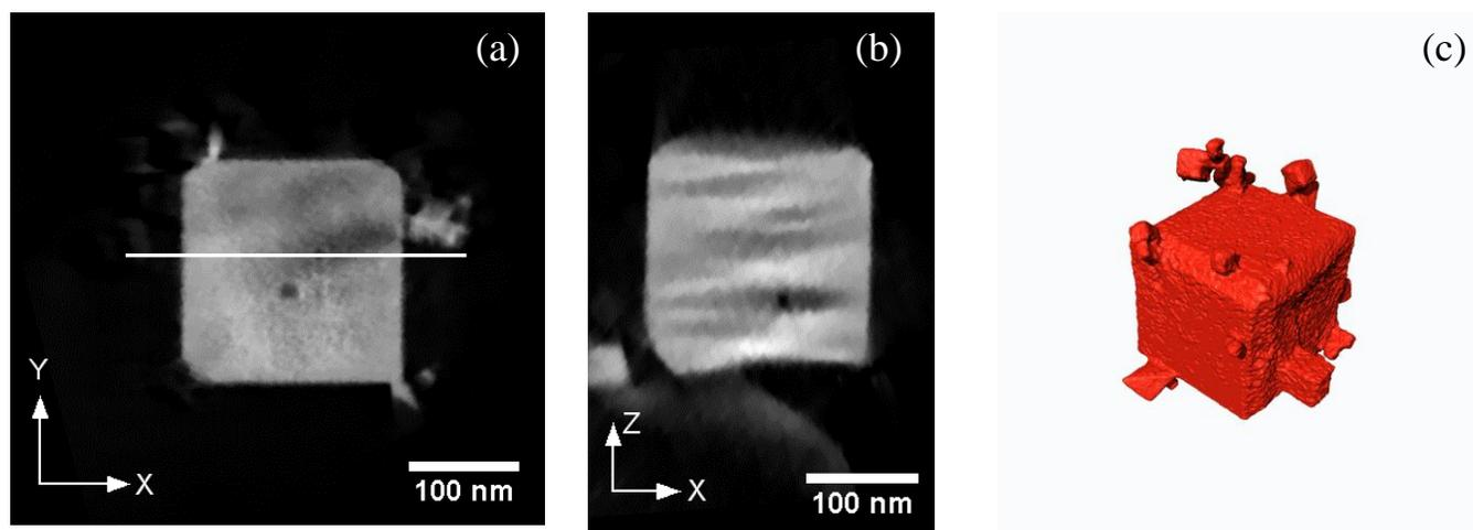
**Figure 1.** Tomographic reconstruction of a MgO smoke cube using the MBIR algorithm from [3]: a single slice in the X-Y plane (a), and in the X-Z plane (b) where the horizontal line in (a) indicates the position of the slice shown in (b), and a 3D perspective view of the particle after segmentation (c).
