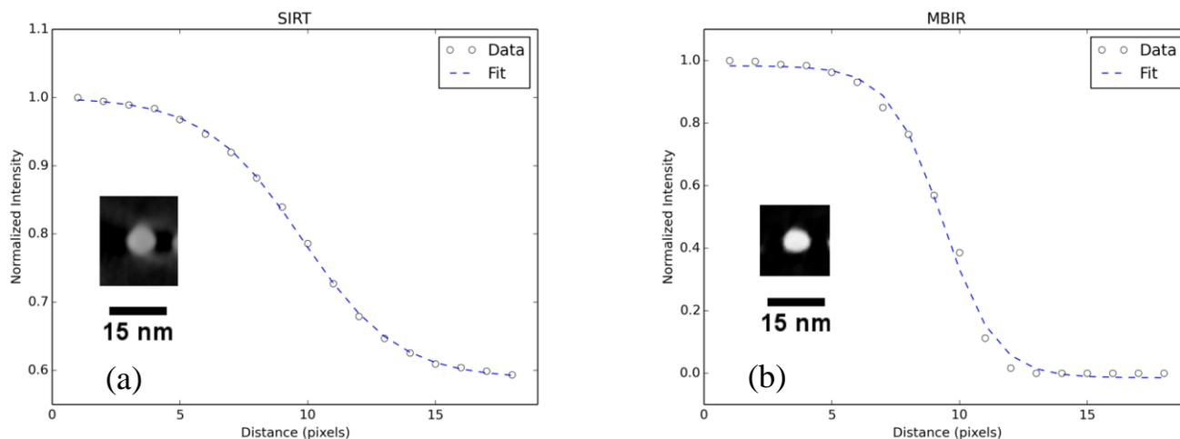
**Figure 2:** Results of curve fitting to edge intensity profiles along the z direction (optical axis) from tomographic reconstructions of the same Au particle using two different reconstruction methods. 141 ADF-STEM images acquired at  $1^\circ$  tilt intervals from  $-70^\circ$  to  $+70^\circ$  were used for the reconstruction.
