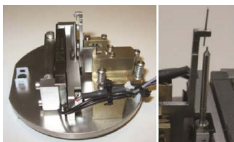
Figure 1. Optical picture of the custom load cell (Left) and a magnified view of the load cell in uniaxial compression mode before fine alignment.
