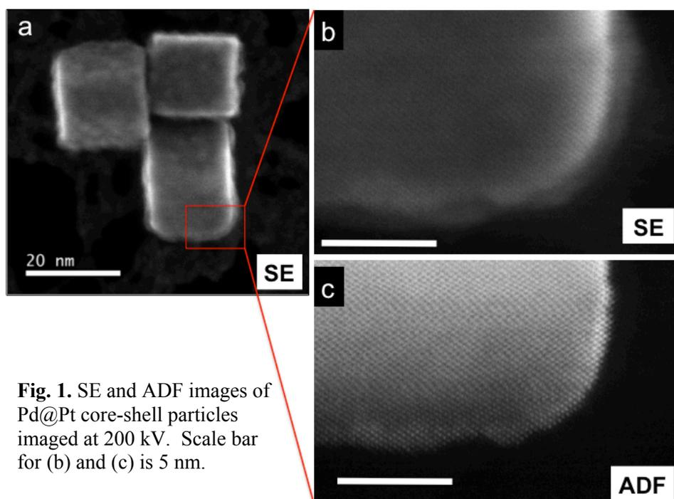
**Fig. 1.** SE and ADF images of Pd@Pt core-shell particles imaged at 200 kV. Scale bar for (b) and (c) is 5 nm.
