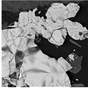
**Figure 1:** Rutherford backscattered ion image of band gap variation in a cleaved MoS<sub>2</sub> sample using a 37 kV He ion.
