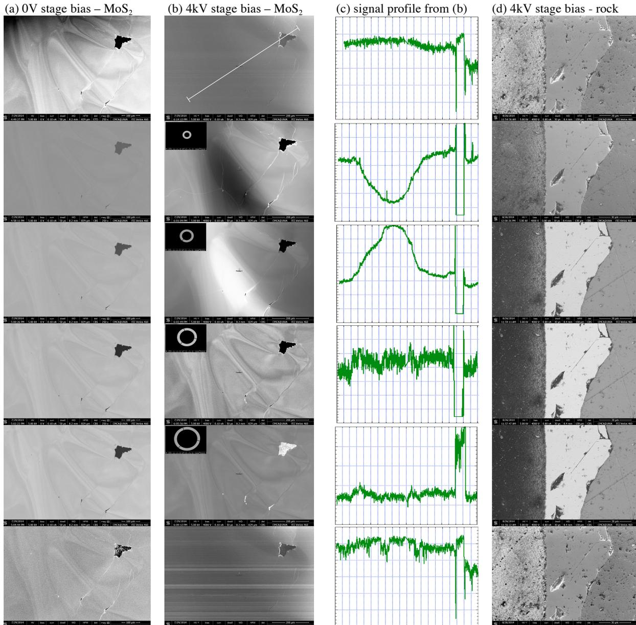
**Figure 3:** From top: ET-SE, DBS-A, DBS-B, DBS-C, DBS-D and TLD images of biased (4kV) and unbiased cleaved MoS<sub>2</sub> and a polished rock sample (with vertical carbon ink line down the left-hand side) together with the signal profile along the line shown in the top ET-SEI from the biased condition.
