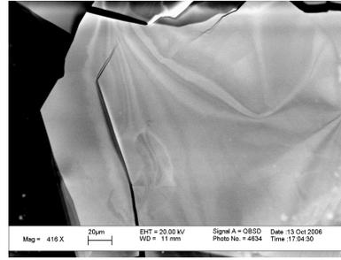
**Figure 2:** BSEI of band gap variation in the same cleaved MoS<sub>2</sub> sample using a conventional FESEM at 20 kV.
