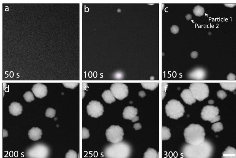
**Figure 1.** a-f) Time-lapsed ADF STEM images showing the electron beam induced nucleation and growth of Pt from a 1 mM  $\text{K}_2\text{PtCl}_6$  + 0.5 M  $\text{H}_2\text{SO}_4$  solution. The electron dose rate is  $196 \text{ e}^-/\text{nm}^2\text{s}$  and the scale bar is 200 nm.
